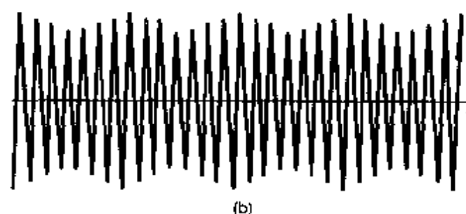
Figure 8.34 Comparison of narrowband FM and AM-DSB/SC: (a) narrowband FM; (b) AM-DSB/SC.
